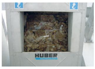
STEP SCREEN® Flexible: very high operational stability and reliable operation without impairment by grit, gravel and stones due to the special bottom step design for lifting of screenings at bottom level.
