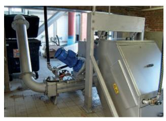
STEP SCREEN® Flexible combined with HUBER Wash Press type SL for intensive screenings washing. Totally enclosed, odour-free design.
