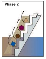
The complete screenings carpet is lifted and transported by rotation of the moveable lamella unit.
