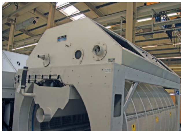
Polyurethane sealing in the inlet of the HUBER Drum Screen LIQUID
