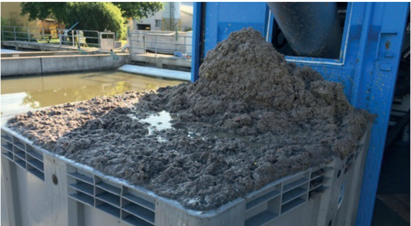
Screenings separated by the HUBER Drum Screen LIQUID mesh: The load to be handled in the biological treatment stage is reduced and more gas can be produced in the digester.
