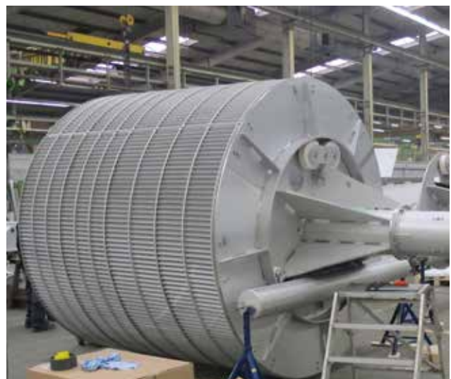
HUBER Perforated Plate Screen ROTAMAT® STAR, 2600 mm diameter, 1 mm perforation.
